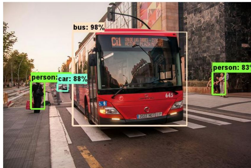
Figure 6. Example objection detection results using MobileNet SSD.
